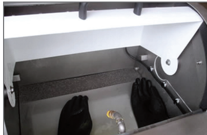
Hot water spray washer to debond part and fixture in hot water soak tub.
