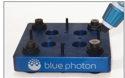
Handheld pressurized steamer to remove residual adhesive from grippers and workpieces.
